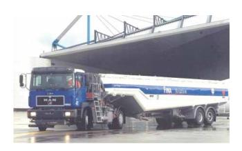
Esterer Aircraft Refueller type FTS is designed to service all aircrafts with overwing and underwing reel and deck hoses.
